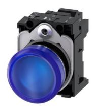
Indicator lights, 22 mm, round, Metal, shiny, blue, lens, smooth, with holder, LED module with integrated LED 230 V AC, spring-type terminal, with laser labeling, upper case and lower case, always upper case at beginning of line
