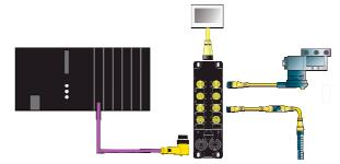
Contained in a 60mm wide housing rated for IP67 environments, BradControl I/O modules can be machine mounted and are able to withstand areas where liquids, dust or vibration may be present. This makes them ideally suited for many applications including material handling equipment and automated assembly machinery.
