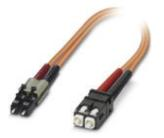
Assembled FO cable, zip cord cable, multi-mode fiberglass 50/125  $\mu$ m, OM2, plug: LC/SC-RJ, degree of protection: IP20, for installation in cable ducts or control cabinets, length: 2 m
