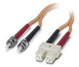
Assembled FO cable, zip cord cable, multi-mode fiberglass  $50/125 \mu m$ , OM2, plug: SC duplex/B-FOC (ST), degree of protection: IP20, for installation in cable ducts or control cabinets, length: 2 m
