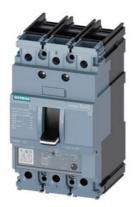
circuit breaker 3VA5 UL frame 125 breaking capacity class S 25kA @ 480 V 3-pole, line protection TM230, FTAM, In=25A overload protection Ir=25A fixed short-circuit protection Ii=6...12 x In UL489 SB (naval), 50 deg. cel. cable connection on both sides
