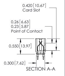
Note: MBB switching contacts assembled in specified positions are available on request. 717 Series Ultra-Mate Card Edge Connector - Press Fit Part Number: 717-064-520-201
