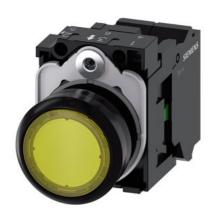
Illuminated pushbutton, 22 mm, round, plastic, yellow, pushbutton, flat, momentary contact type, with holder, 1NO, LED module with integrated LED 24 V AC/DC, spring-type terminal, with laser labeling, upper case and lower case, always upper case at beginning of line
