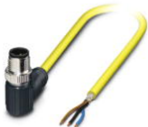
Sensor/actuator cable, 3-position, PVC, yellow, shielded, Plug angled M12 SPEEDCON, A-coded, on free cable end, cable length: 2 m
