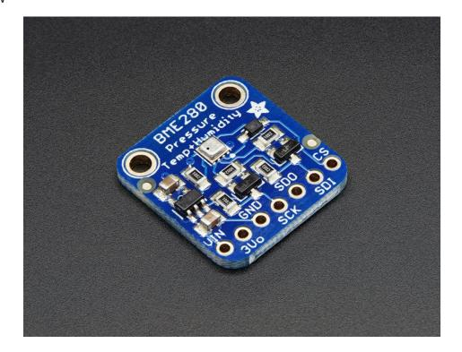
Bosch has stepped up their game with their new BME280 sensor, an environmental sensor with temperature, barometric pressure *and* humidity! This sensor is great for all sorts of weather/environmental sensing and can even be used in both I2C and SPI!
