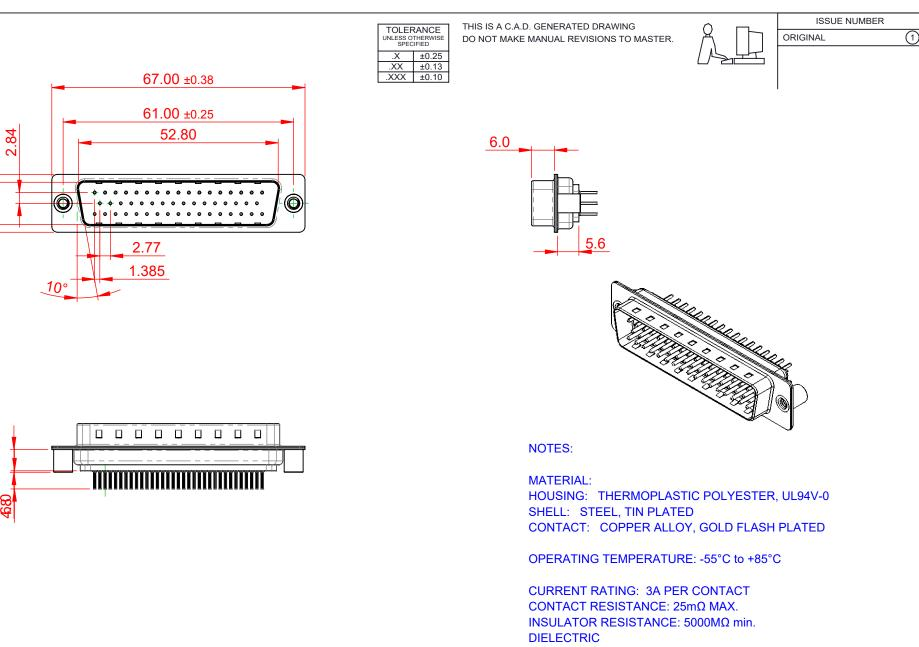
WITHSTANDING VOLTAGE: 1000V AC rms
