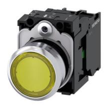
Illuminated pushbutton, 22 mm, round, metal, shiny, yellow, pushbutton, flat, momentary contact type, with holder, 1NO, LED module with integrated LED 110 V AC, screw terminal, with laser labeling, upper case
