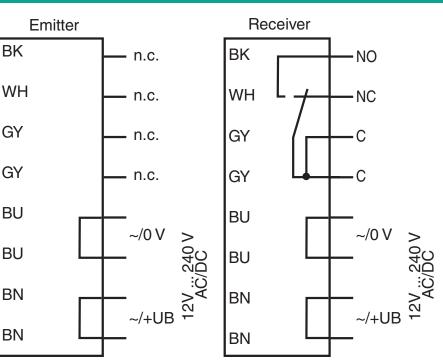
The relay-functions "NC" and "NO" bear on the switching mode "Dark-ON". This complies to the default setting of the light/dark switch (factory setting).
