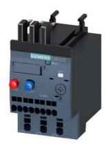
Overload relay 0.90...1.25 A Thermal For motor protection Size S00, Class 10 Contactor mounting Main circuit: Spring-type terminal Auxiliary circuit: spring-type terminal Manual-Automatic-Reset
