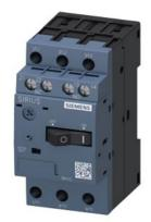
Circuit breaker size S00 for motor protection, CLASS 10 A-release 0.9...1.25 A N-release 16 A 1 NO+1 NC transverse Screw terminal Standard switching capacity
