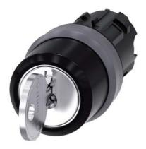
RONIS key-operated switch, 22 mm, round, plastic with metal front ring, lock number SB30, with 2 keys, 3 switch positions I-O-II, latching, actuating angle 2x45°, 10:30h/12h/13:30h, Key removal I+II, possible special locks: SB31, 421, 455, with laser labeling, inscription or symbol Customer-specific selection with SIRIUS ACT configurator (CIN)
