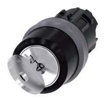
RONIS key-operated switch, 22 mm, round, plastic with metal front ring, lock number 455, with 2 keys, 2 switch positions O-I, latching, actuating angle  $90^\circ$ , 10:30h/13:30h, key removal O, with laser labeling, upper case and lower case, always upper case at beginning of line
