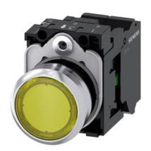
Illuminated pushbutton, 22 mm, round, metal, shiny, yellow, pushbutton, flat, momentary contact type, with holder, 1NO, LED module with integrated LED 24 V AC/DC, spring-type terminal, with laser labeling, inscription or symbol Customer-specific selection with SIRIUS ACT configurator (CIN)
