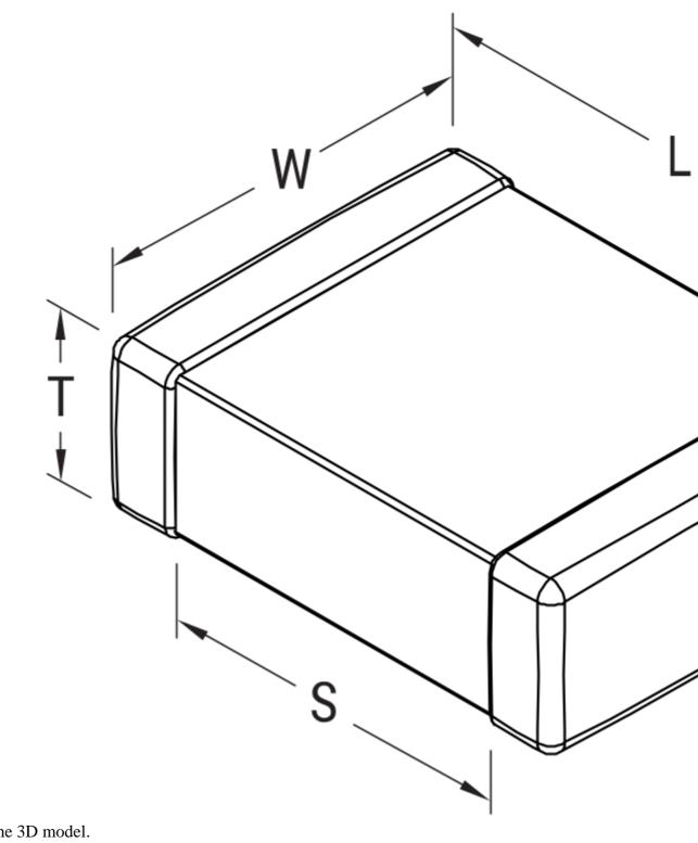
Click <u>here</u> for the 3D model. Dimensions Chip Size 0805 L 2mm +/-0.2mm
