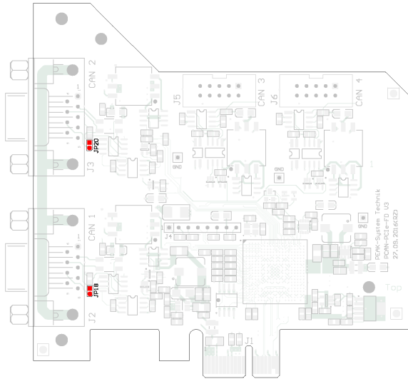
Position of the solder fields on the top side of the card for the activation of the daisy chain
