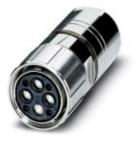
Cable connector, straight, Screw locking, M58, number of positions: 4+3+PE, type of contact: Socket, Crimp connection, shielded: yes, cable diameter range: 17 mm ... 25 mm
