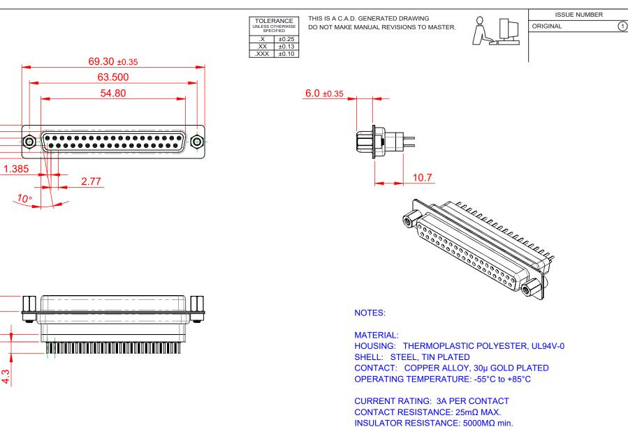
DIELECTRIC WITHSTANDING VOLTAGE: 1000V AC rms
