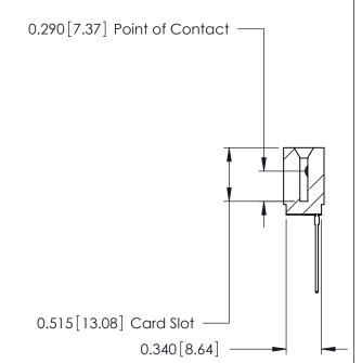
ACAD REFERENCE NO. 746 Series Ultra-Mate Card Edge Connector - Press Fit DRAWN: J.LEE Part Number: 746-022-541-101 CHECKED: **EDAC INC** SCALE: THESE DRAWINGS AND SPECIFICATIONS ARE THE PROPERTY OF EDAC INC., AND TORONTO, ONTARIO SHALL NOT BE REPRODUCED, OR COPIED DRAWING NUMBER CANADA OR USED AS THE BASIS FOR THE 746-ENG MASTER MANUFACTURE OR SALE OF APPARATUS YOUR CONNECTION TO QUALITY & SERVICE WITHOUT WRITTEN PERMISSION.
