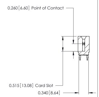
ACAD REFERENCE NO. 746-ENG MASTER 746 Series Ultra-Mate Card Edge Connector - Press Fit DRAWN: J.LEE DATE: AUG 20/09 Part Number: 746-050-520-201 CHECKED: DATE: **EDAC INC** SCALE: SHEET 1 OF 1 THESE DRAWINGS AND SPECIFICATIONS ARE THE PROPERTY OF EDAC INC.,AND TORONTO, ONTARIO SHALL NOT BE REPRODUCED, OR COPIED DRAWING NUMBER CANADA OR USED AS THE BASIS FOR THE 746-ENG MASTER MANUFACTURE OR SALE OF APPARATUS YOUR CONNECTION TO QUALITY & SERVICE WITHOUT WRITTEN PERMISSION.
