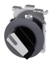
Selector switch, illuminable, 30 mm, round, Metal, matte, white, selector switch, short, front ring for flush installation, 2 switch positions O-I, latching, actuating angle  $90^\circ,\,10:30h/13:30h,$  with laser labeling, upper case and lower case, always upper case at beginning of line
