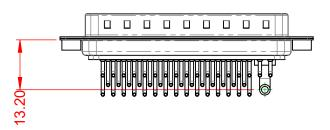
POWER/CO-AX CONTACT RATING:20A (CURRENT)(IF PRESENT)SIGNAL CONTACT CURRENT RATING:5A PER CONTACTSIGNAL CONTACT RESISTANCE: $10m\Omega$  MAX.INSULATOR RESISTANCE: $5000M\Omega$  min.DIELECTRIC $5000M\Omega$  min.
