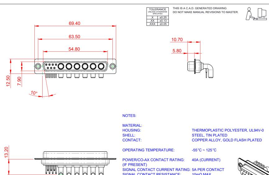
SIGNAL CONTACT CURRENT RATING: 5A PER CONTACT SIGNAL CONTACT RESISTANCE:  $10m\Omega$  MAX.
