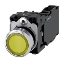
Illuminated pushbutton, 22 mm, round, Metal, shiny, yellow, pushbutton, flat, momentary contact type, with holder, 1 NO+1 NC, LED module with integrated LED 230 V AC, screw terminal, with laser labeling, upper case
