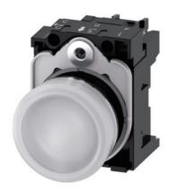
Indicator lights, 22 mm, round, Metal, shiny, white, lens, smooth, with holder, LED module with integrated LED 230 V AC, screw terminal, with laser labeling, upper case and lower case, always upper case at beginning of line
