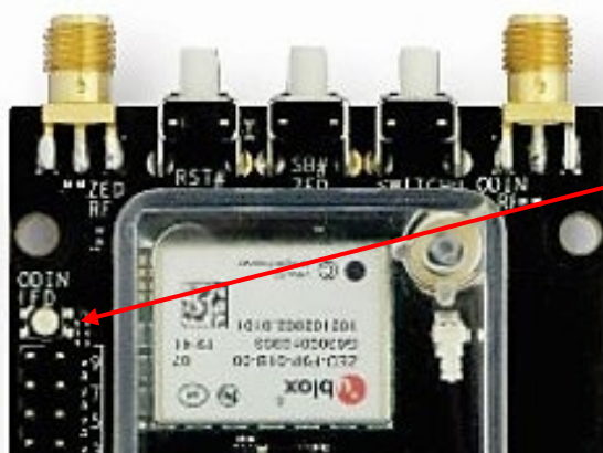
Figure 8: ODIN-W2 activity LED position on C099-F9P board
