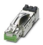
RJ45 connector, degree of protection: IP20, number of positions: 8, 10 Gbps, material: Zinc die-cast, connection method: IDC, connection cross section: AWG 23- 22, cable outlet: straight, High degree of resistance to vibration; 360° shielding; one-piece design; special tool-free assembly
