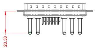
20A (CURRENT) POWER/CO-AX CONTACT RATING: (IF PRESENT) SIGNAL CONTACT CURRENT RATING: 5A PER CONTACT SIGNAL CONTACT RESISTANCE:  $10m\Omega$  MAX. **INSULATOR RESISTANCE:** 5000MΩ min. DIELECTRIC
