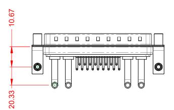
OPERATING TEMPERATURE: $-55^{\circ}C \sim 125^{\circ}C$ POWER/CO-AX CONTACT RATING:30A (CURRENT)(IF PRESENT)SIGNAL CONTACT CURRENT RATING:5A PER CONTACTSIGNAL CONTACT RESISTANCE: $10m\Omega$  MAX.INSULATOR RESISTANCE: $5000M\Omega$  min.DIELECTRIC $5000M\Omega$  min.
