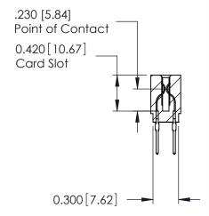
ACAD REFERENCE NO ECTION SARA 725 Series Ultra-Mate Card Edge Connector - Press Fit Part Number: 725-052-522-201 **EDAC INC** THESE DRAWINGS AND SPECIFICATIONS ARE THE PROPERTY OF EDAC INC.,AND TORONTO, ONTARIO SHALL NOT BE REPRODUCED, OR COPIED CANADA OR USED AS THE BASIS FOR THE MANUFACTURE OR SALE OF APPARATUS YOUR CONNECTION TO QUALITY & SERVICE WITHOUT WRITTEN PERMISSION.
