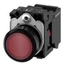
Illuminated pushbutton, 22 mm, round, plastic, red, pushbutton, flat, momentary contact type, with holder, 1NC, LED module with integrated LED 110 V AC, spring-type terminal, with laser labeling, symbol number according to, ISO 7000 or IEC 60417
