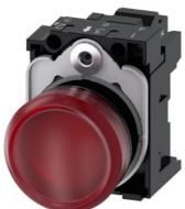
Indicator light, 22 mm, round, plastic, red, lens, smooth, with holder, LED module with integrated LED 110 V AC, spring-type terminal, with laser labeling, upper case and lower case, always upper case at beginning of line
