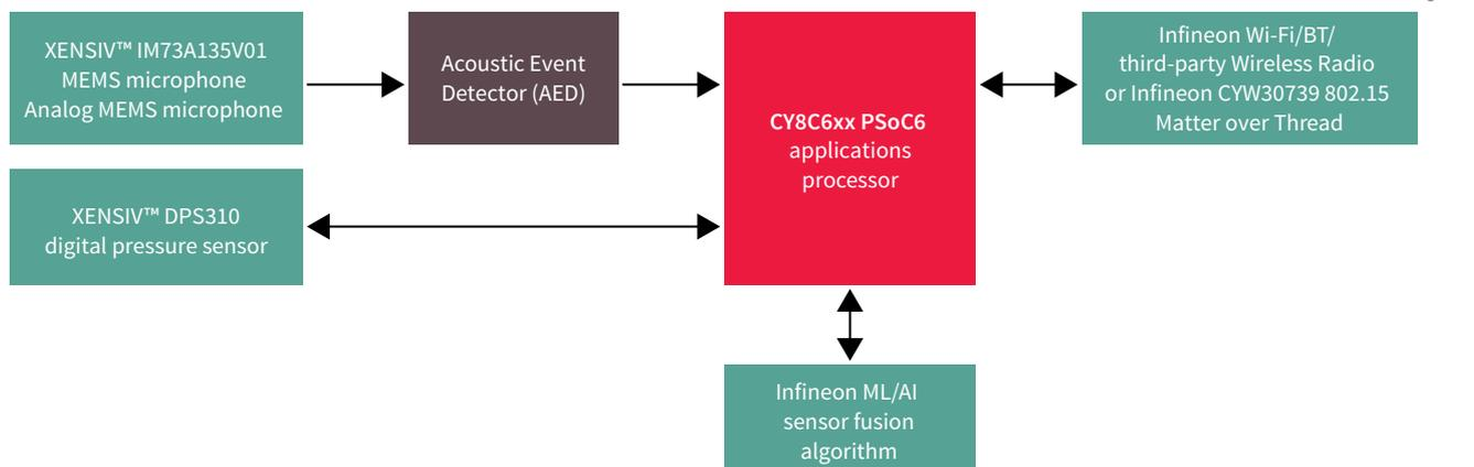
The EVAL\_SEN\_SMART\_ALARM is the evaluation and testing kit for the Smart Alarm System. This kit is shown in the picture below and consists of the following major components
