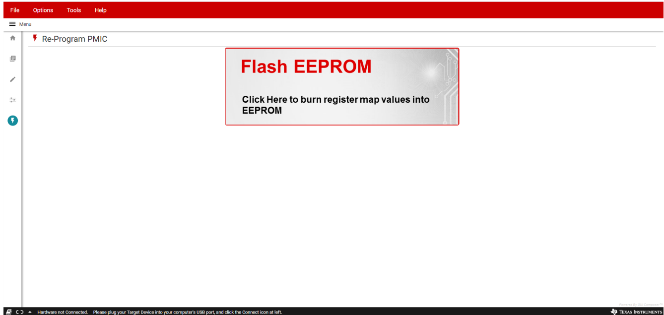
Figure 4-12. TPS6503xx-Q1 GUI Re-Program PMIC Page
