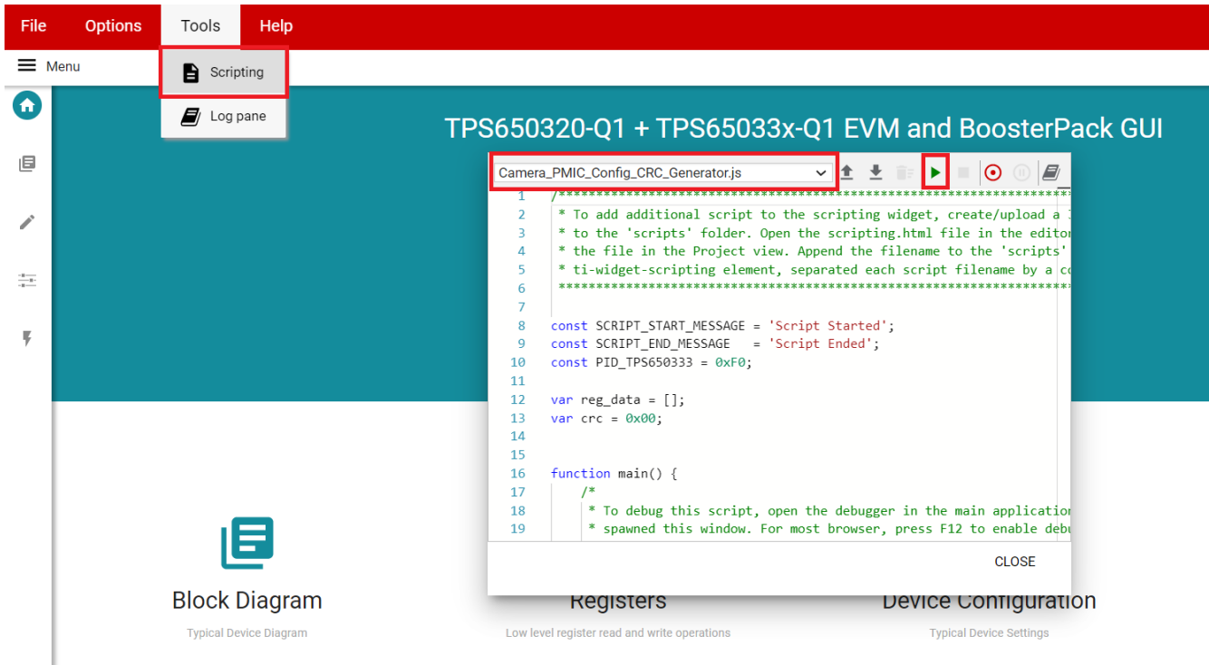
Figure 4-13. GUI Configuration CRC Script
