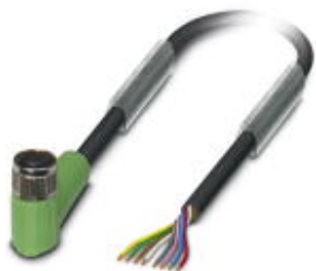
Sensor/actuator cable, 8-position, PUR halogen-free, black-gray RAL 7021, free cable end, on Socket angled M8, cable length: 5 m
