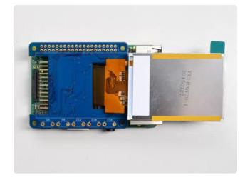
Place the PiTFT HAT on top so all the pins stick through the connector on the side. Gently flip the TFT so its off to the side and wont be in your way while you solder
