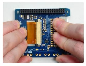
Turn the board over and press gently on the back to get the TFT stuck-on well!
