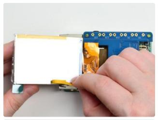
Now we can attach the screen. Remove the two thin tape cover strips.
