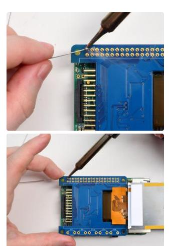
Heat up your soldering iron, and grab some solder. Start by tack-soldering one of the corners. Then you can re-heat that solder point and adjust the circuit board to make it sit flat.
