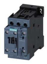
power contactor, AC-3 17 A, 7.5 kW / 400 V 1 NO + 1 NC, 12 V DC, 3-pole, Size S0 screw terminal
