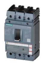
circuit breaker 3VA5 UL frame 250 breaking capacity class C 100kA @ 480 V 3-pole, line protection TM230, FTAM, In=110A overload protection Ir=110A fixed short-circuit protection Ii=5...10 x In nut keeper kit on both sides
