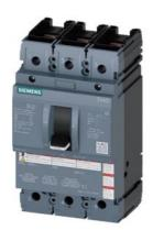
molded case switch 3VA5 UL frame 250 max. sh-circ breaking capacity 65kA @ 480 V 3-pole, line protection MCS110, ln=150A without overload protection self-protection li=16 x ln nut keeper kit on both sides
