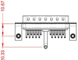
20A (CURRENT) POWER/CO-AX CONTACT RATING: (IF PRESENT) SIGNAL CONTACT CURRENT RATING: 5A PER CONTACT SIGNAL CONTACT RESISTANCE:  $10m\Omega$  MAX.
