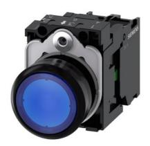
Illuminated pushbutton, 22 mm, round, plastic, blue, pushbutton, flat, momentary contact type, with holder, 1NO, LED module with integrated LED 110 V AC, screw terminal, with laser labeling, upper case
