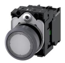
Illuminated pushbutton, 22 mm, round, plastic with metal front ring, clear, pushbutton, flat, momentary contact type, with holder, 1NO, LED module with integrated LED 24 V AC/DC, screw terminal, with laser labeling, inscription or symbol Customer-specific selection with SIRIUS ACT configurator (CIN)
