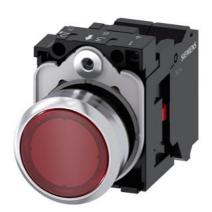
Illuminated pushbutton, 22 mm, round, metal, shiny, red, pushbutton, flat, momentary contact type, with holder, 1NC, LED module with integrated LED 110 V AC, spring-type terminal, with laser labeling, upper case and lower case, always upper case at beginning of line
