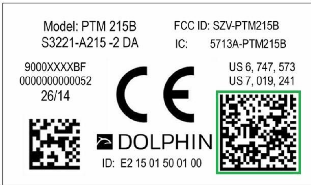
Figure 18 – Location of the commissioning DMC code
