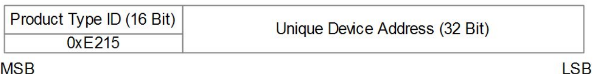
Figure 10 – BLE static source address structure
