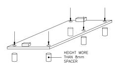
Please leave 4.5mm space from the unit surfaces and leave 4.5mm space from the sides of PCB. For the solder surface, 8mm space is necessary. If the space is not enough, the specification for insulation and withstand voltage will not be satisfied.
