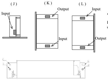
C: 1-Φ4.5 holes and R2.25 slot hole by 2-M4 screws D: Embossed tapped and countersunk holes by 2-M4 screws.
