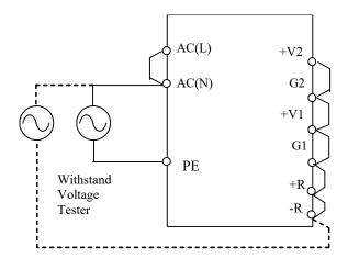
Output ~ PE (Chassis) 500VAC 1min. ( 100mA )
