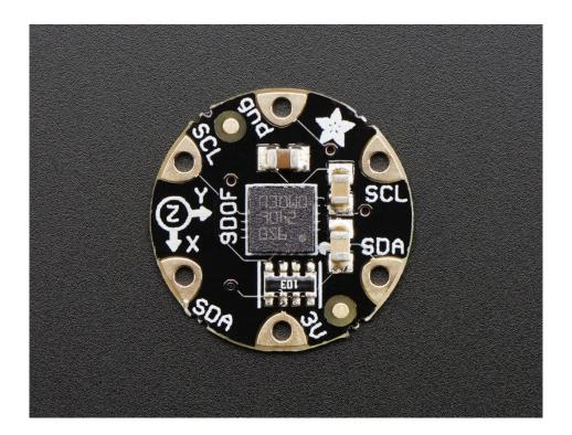
The Flora version has just I2C interface for a super-small design. Attaching it to the FLORA is simple: line up the sensor so its adjacent to the SDA/SCL pins and sew conductive thread from the 3V, SDA, SCL and GND pins. They line up perfectly so you will not have any crossed lines. You can only connect one of these sensors to your FLORA, but you can connect other I2C sensors/outputs by using the set of SCL/SDA pins on the opposite side.
