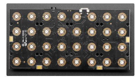
The NeoPixels are chained together, and connect in a zig-zag. The first pixel is in the top left, the last pixel is on the bottom right. In Arduino, the NeoPixels are on pin 10, in CircuitPython they are on on board.NEOPIXEL
