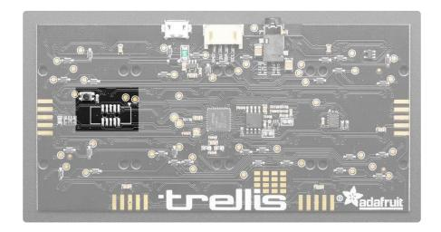
There's a small reset button on the back of the PCB, you can double-click it to enter the bootloader.
