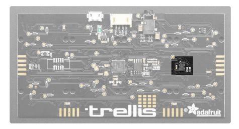
This sensor is on a separate I2C port, which is available in Arduino under Wire1 or in CircuitPython under <a href="mailto:board.ACCELEROMETER\_SCL">board.ACCELEROMETER\_SCL</a> and <a href="mailto:board.ACCELEROMETER\_SDA">board.ACCELEROMETER\_SDA</a>
